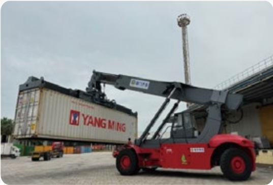
Picture: The first front-loader converted from oil into electricity in Fujian Province ▶
