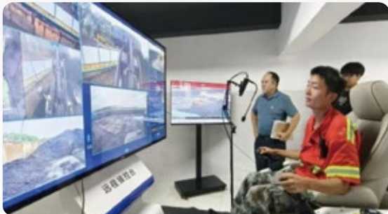
▲ Picture: 5G electric loader remote control operating room
